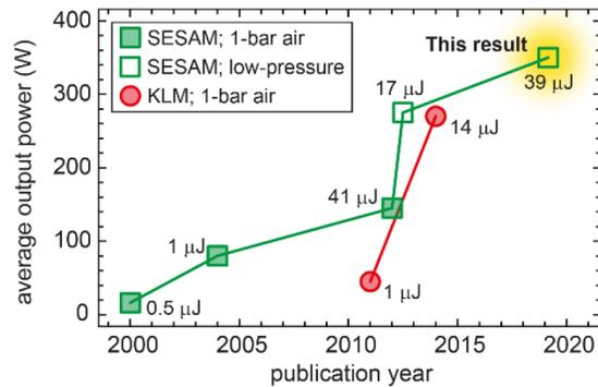
**Fig. 1.** Average output power from Yb:YAG SESAM-modelocked and KLM oscillators, which represented a new record at the time of publication. The labels indicate the output pulse energy. References are provided in the text. In this result we combine a cavity design including multiple reflections on the disk gain medium with operation in a low-pressure environment.
