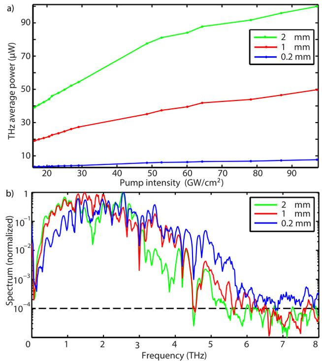
**Figure 2.** (a) Power of the generated THz pulses versus the peak intensity of pump pulses for different thicknesses of GaP, obtained under ambient conditions. (b) Power spectra of the generated THz pulses at  $97 \text{ GW}/\text{cm}^2$  pump peak intensity for different thicknesses of GaP.
